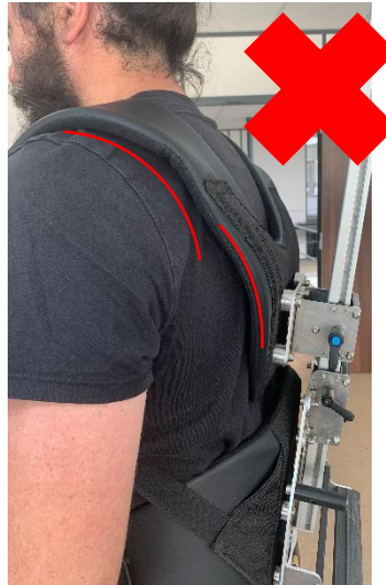
Figure 2: Shoulder harness positioned too low. The curvature of the harness does not hug the shoulder
