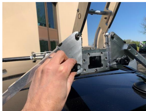
Figure 7: Adjust the trim by adjusting the angles of the two side arms using the rear knobs
