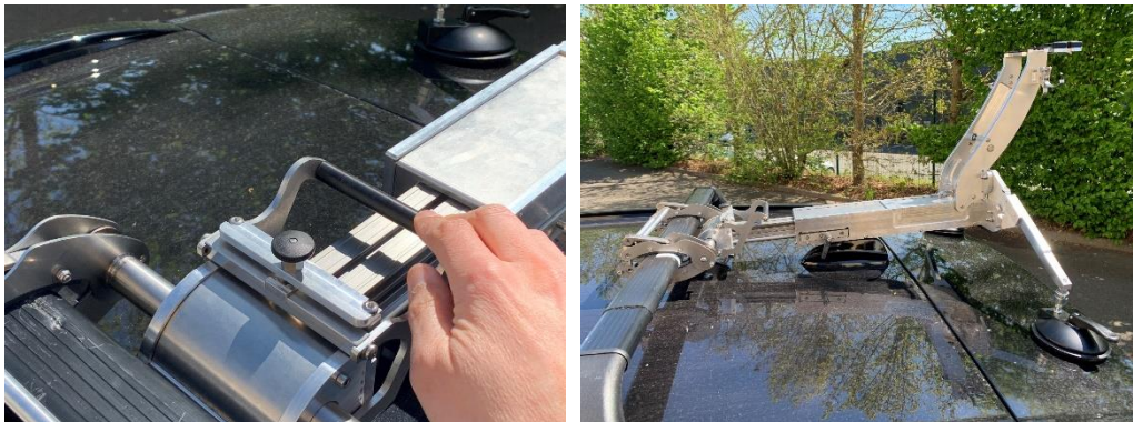
Figure 6: Close the jaw and make sure the pin is engaged
