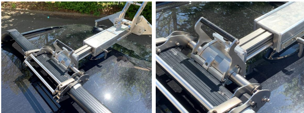
Figure 5: Engage the front jaw on the clamp
