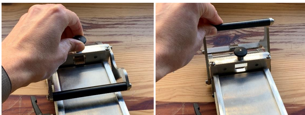
Figure 3: Lift the pin and open the jaw forward
