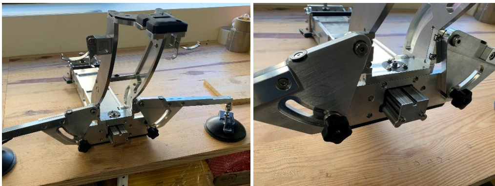
Figure 2: Unfold both arms of the suction cups and tighten the knobs in the groove
