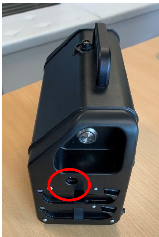
Figure 9: Connectors for 19V external power supply for vehicles
